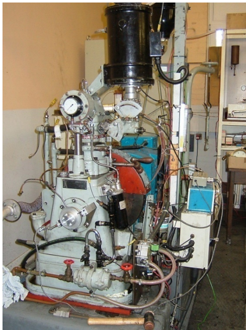
Fig. 15. Experimental set up on a Ricardo E6 engine and an electric dynamometer,
